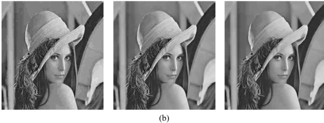
Fig. 2. Comparison between different image coding standards: (a) rate distortion curves and; (b) subjective views at 0.225 bpp (left: JPEG, middle: JPEG 2000 DWT53, right: H.264/AVC I-Frame CAVLC).
